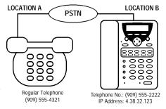
When making a call from location A to location B Simply dial "5552222". Regular Phone on location B will ring. Pick up handset and you can begin communication.
